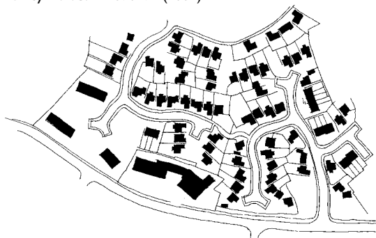
Fig 4. Plan of cul-de-sac design that increases segregation and reduces interaction of communities and surroundings.
