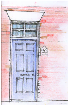
Typical panelled door with fanlight over and rendered feature lintel over
