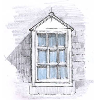
Full dormer with Georgian style window using timber astragals in a slate main roof and lead apron detail
