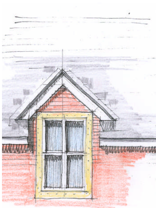
Typical half dormer detail from local village using painted barge boards with apex finial in timber, slate roof and casement window.
